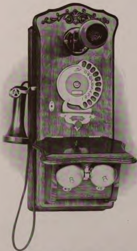
FIG. 3.—AUTOMATIC TELEPHONE WALL SET, SUBSCRIBER'S STATION.
